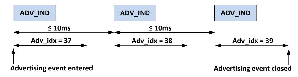
Two subsequent advertising packets within one Adv. Event must be less than 10 ms apart. A mimimum time is not specified.
