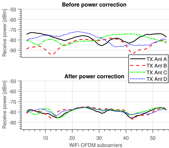
Fig. 6. Receive power of each antenna path at node13-13 before and after power correction respectively.
